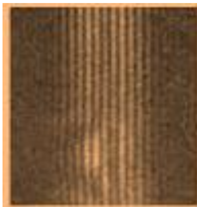
Fig. 11.3: Interference pattern formed by Fresnel's bi-prism.
