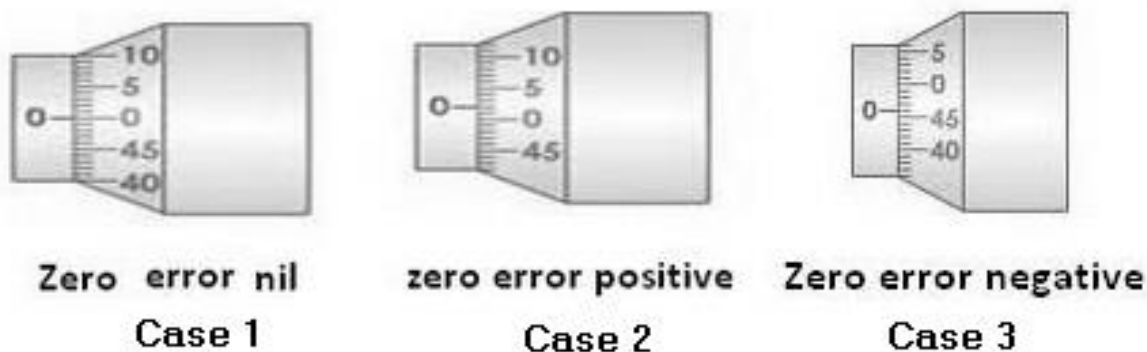
Fig. 1b.2: Analysis of zero error for a screw gauge
