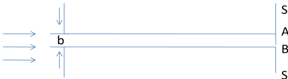
Fig. 5.1: If a plane wave is incident on an aperture then according to geometrical optics a sharp shadow will be cast in the region AB of the screen.
