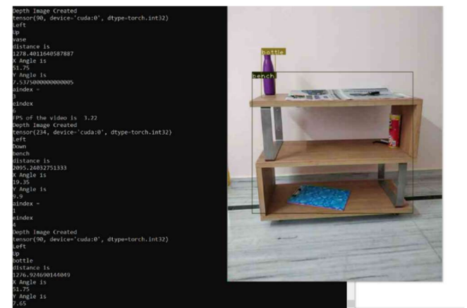
Figure 5.1 Bottle is detected to the left of the user and a spatial audio is generated.
