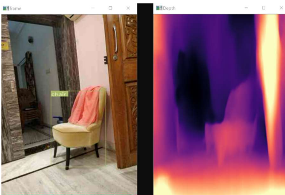
Figure 4. Sample Image and Disparity map obtained for IP Webcam Feed (Left to Right)
