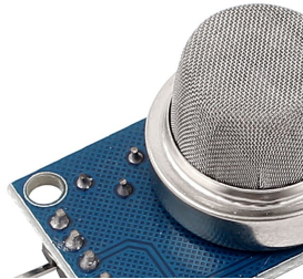
(Fig5. Smoke Sensor)
