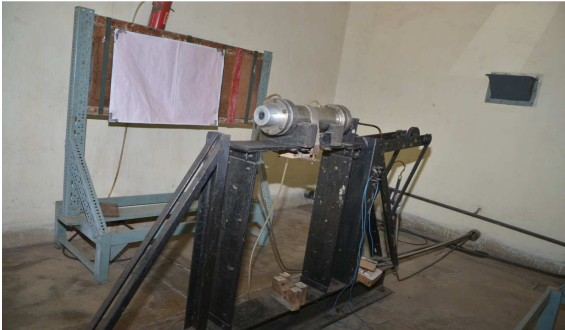
Static test facility for hybrid rocket motor: This facility enables us to get regression rate, pressure of combustion chamber and thrust during the operation of hybrid rocket motor.
