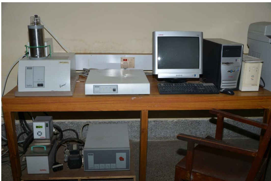
Instrumental facility: It enables us to get thermal decomposition behavior, heat flow and transition temperature various ingredients of propellants at different condition.
