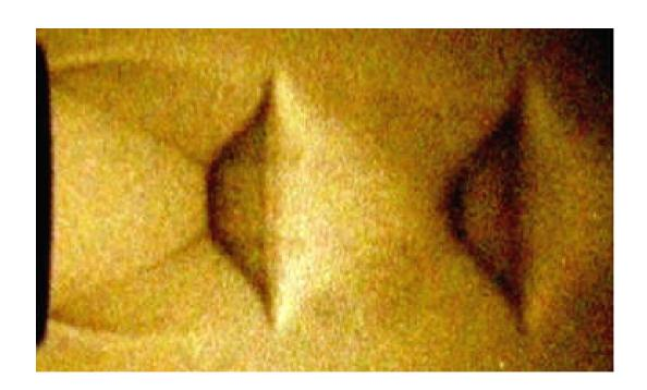
Colored Schlieren visualization of shock structures in a freely expanding jet
