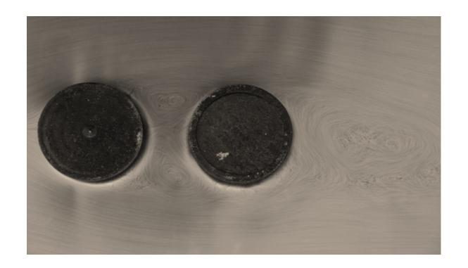
Water tunnel and asymmetric wake flows visualized using water tunnel
