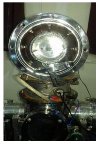
Heater placed inside the vacuum chamber
