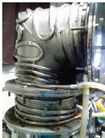
Copper pipe surrounding the heating chamber for cooling
