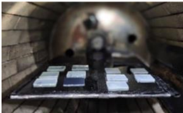
Thin film samples inside the chamber on sample stage holder.
