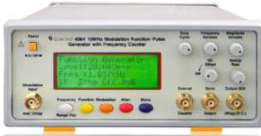
Fig. 2: The function generator used in Physics Laboratory.
