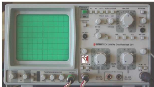
Fig. 3.1- The Cathode ray oscilloscope & frequency generator used in Physics Laboratory
