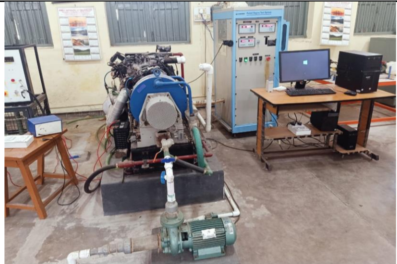
Computerized petrol engine test-rig with eddy current dynamometer.
