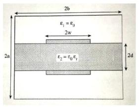
Where a=b=2.5 cm, d=0.5,  $\omega=1 cm$ ,  $\epsilon_1=\epsilon_0$ ,  $\epsilon_2=2.35\epsilon_0$  and the thickness of the strip is neglected. The potential difference applied between the outer metal shield and the inner strips is  $V_d=100 mV$ .
