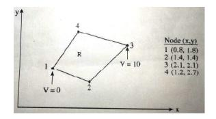
**EXP 12** Solve La Place equation inside the region R as shown in the figure by Finite Element Method (FEM).
