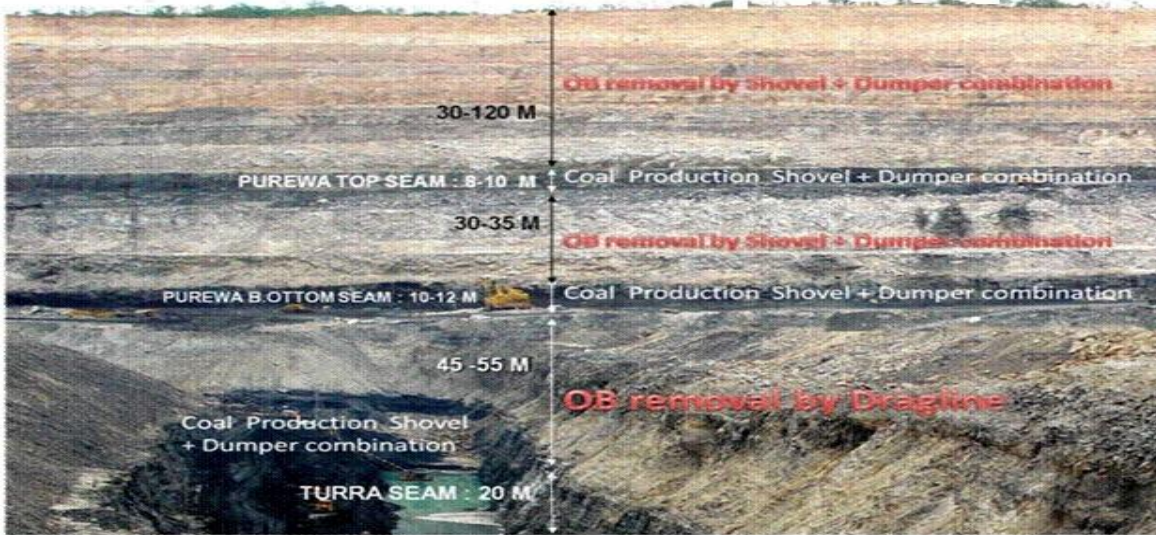
Fig 1: Geological cross-section of an opencast mine
