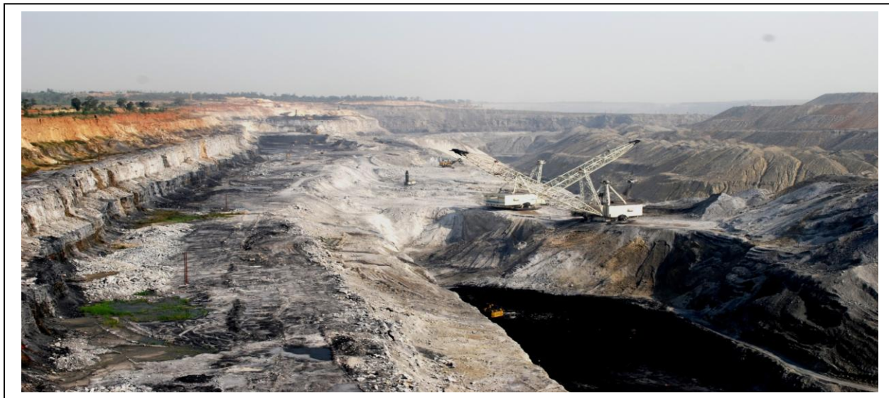
Figure 2: Deployment of dragline and shovel-dumper at different strata
