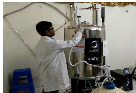
400 MHz Superconducting Magnet of an NMR Laboratory at Department of Chemistry, BIT Mesra, Ranchi
