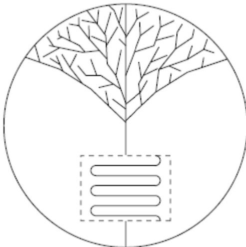
Figure 7.35. Spherulitic structure shown schematically: (1) radial growth and branching of the lamellae, (2) portion of a lamellae enlarged to indicate a folded chain structure showing chain axis perpendicular to the radius of the spherulite
