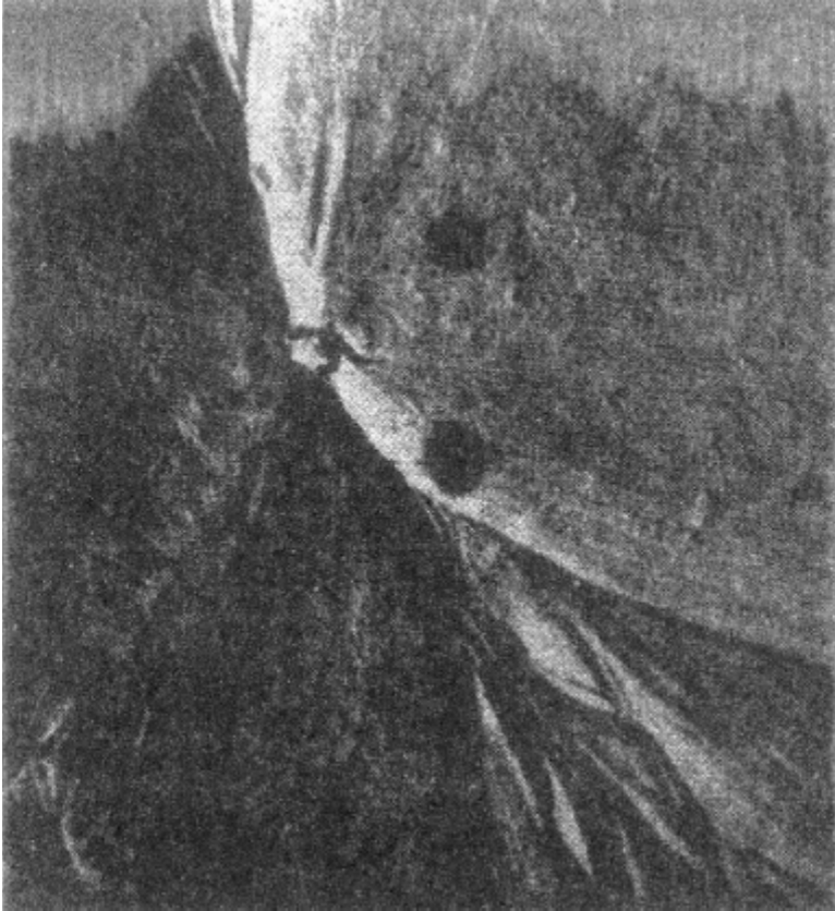
Figure 7.32. Electron micrograph of the surface of polyoxymethylene crystallized by melt cooling 15,16 (Geil, 1960; Courtesy, Wiley-Interscience, New York)
